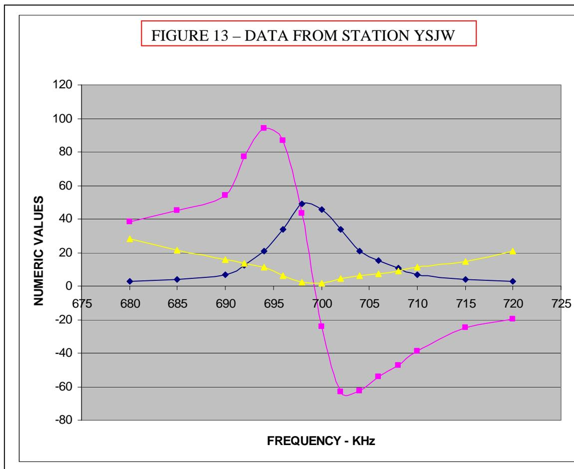
The blue curve is the radiation resistance, the red curve is the reactance, and the yellow curve is the VSWR. For the plot the calculated VSWR was multiplied by 10 to allow readability on the graph. A VSWR value of 20 on the curve represents a true VSWR value of 2:1. From the curve the 2:1 VSWR range is from 685 to 720, approximately 35 KHz.
