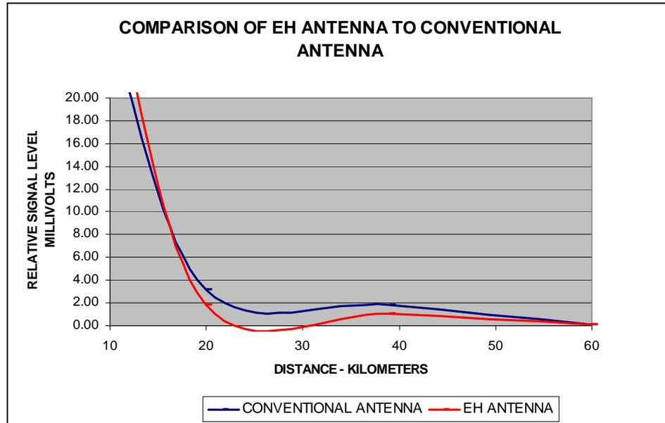
The plot comparing the radiation from the two antennas indicates a cross over at about 16 km. This can be explained by the fact that the pattern from the antenna on the hill actually does not allow signal at close range due to the radiation pattern being blocked by the hill. However, placement on the top of the hill gives an advantage at longer range.
