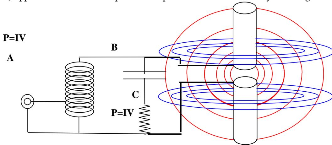
FIGURE 11 - THE INHERENT DETAILS OF AN EH ANTENNA
