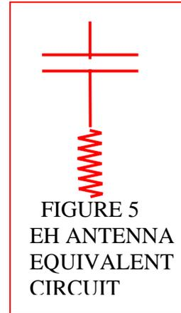
To be able to pass current through the radiation resistance it is necessary to cancel the reactance of the capacitor. This may be done by adding a series inductance having the same value of reactance as the capacitor at the desired operating frequency. This creates a series resonant circuit as shown in Figure 6. The inductor (coil) can be tapped to provide a convenient 50 ohm match to allow use of a coaxial transmission line. The complete antenna is depicted in Figure 7.
