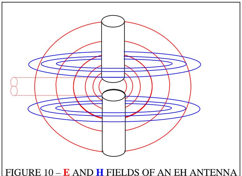
**FIGURE 10 – E AND H FIELDS OF AN EH ANTENNA**
