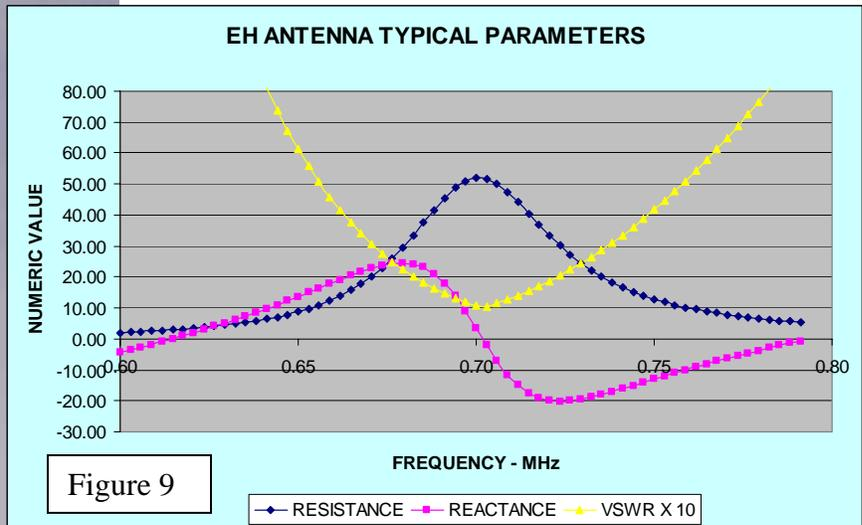
The reactive component of the input impedance goes from + through 0 at the design frequency then to - at higher frequencies.
